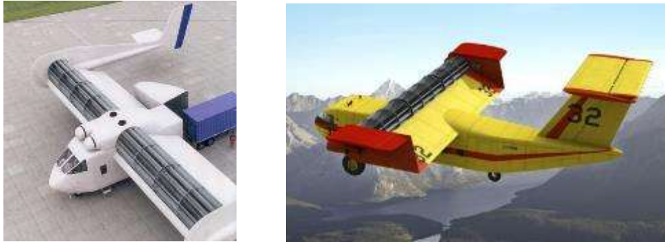
Figure 80: Advanced small aircraft using the fan-wing concept
